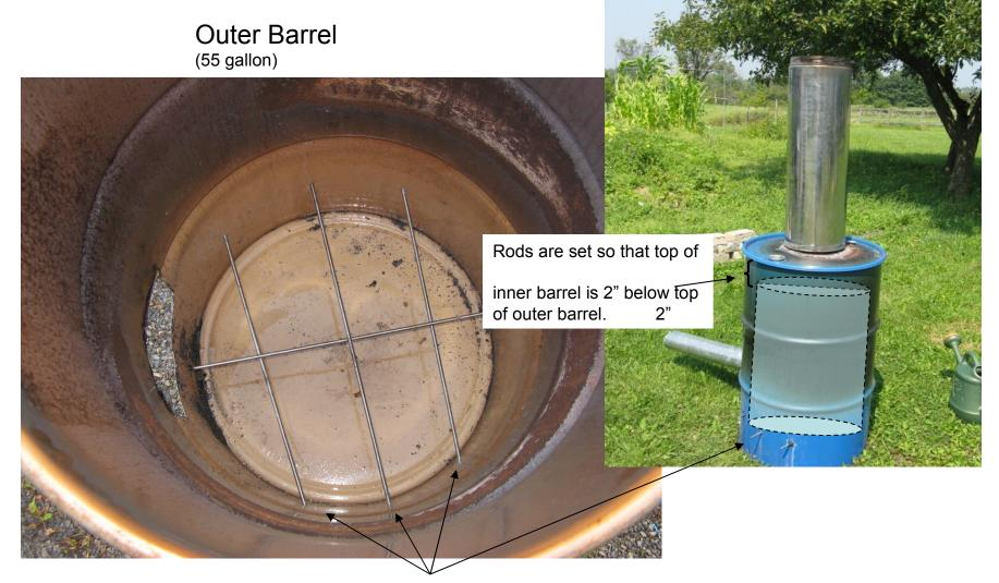
Rods support inner barrel.
