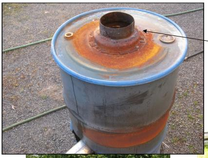
Stove pipe flange with 6" hole in barrel lid
