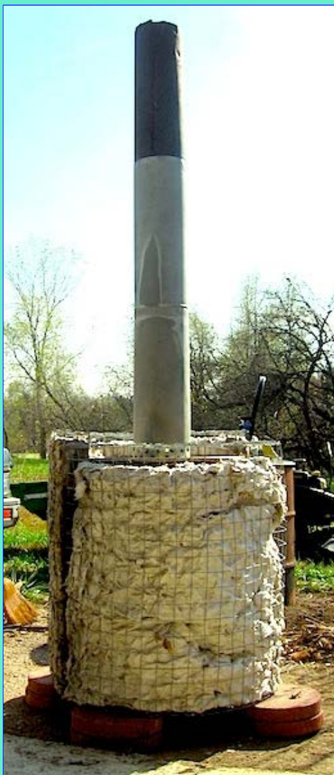
55-gallon Barrel Burner with weathered fiberglass insulation
